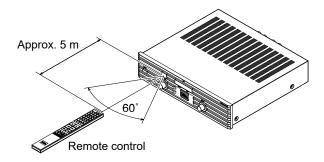
Operate the remote control within approx. 5 m distance from the front panel of the main unit within an angle of 60° to the remote sensor.
